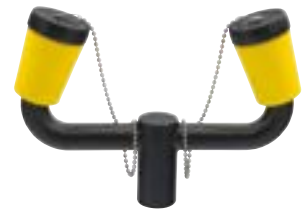
Model 01052111 Eyewash Assembly with ABS Heads, Wye & Covers, SS bead chain, 1/2" / 1.3 cm Inlet, 0.4 gpm / 1.5 lpm, for self contained portable
